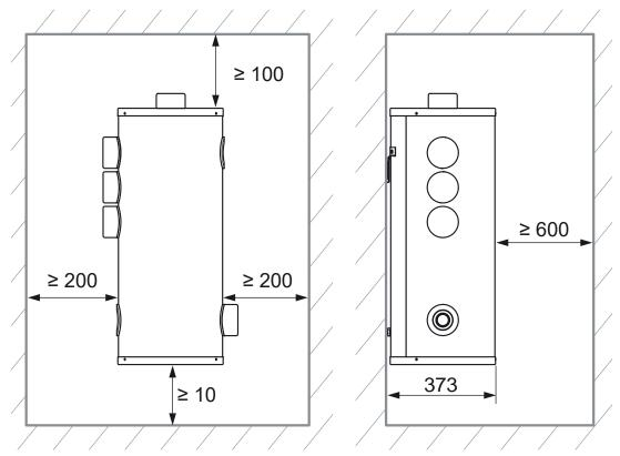
NOTE: All measurements are millimetres. Clearance necessary for the installation or maintenance of the appliance
