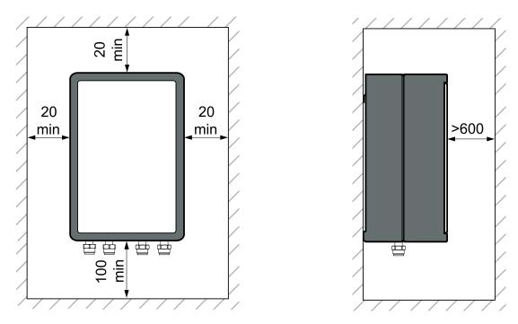
NOTE: All measurements are millimetres. Clearance necessary for the installation or maintenance of the appliance
